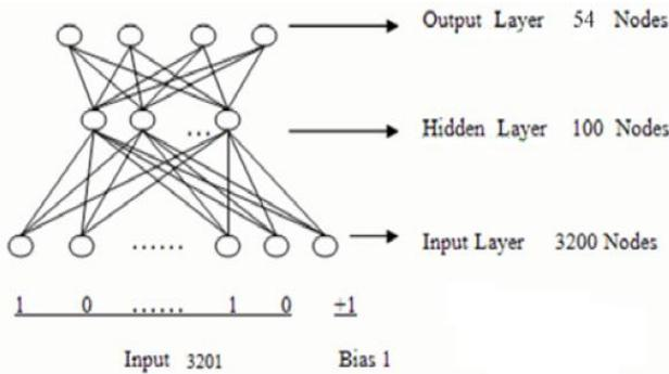
Fig. 4. Three-layer back-propagation neural network.
